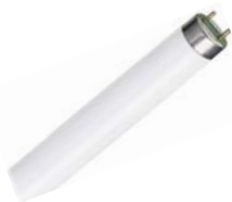
HYZT18DL (H139) TRIFOSFORO T8 6500K, G13, 18W, 1250LUMS, 10000HRS, 604LONG, 26Ø
