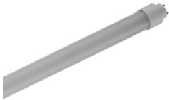
NL-10W-T8-2FT (N002) 10W =18W, BALASTRO 1.7G, 860LUMS, 5500k - 6500k, 600 LONG, 30Ø, Blanco Mate, 55Ø
